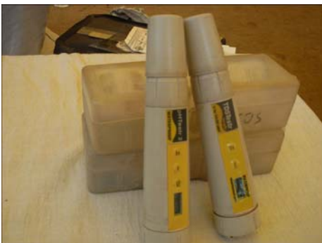
TDS Meter and Ph Meter
